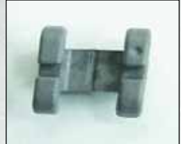
A "green state" bracket is produced
